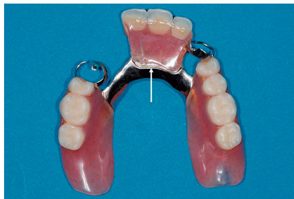
Fig. 6 Lack of bonding at the metal–resin interface in the anterior region resulted in loosening of the denture base from the framework (arrow).
