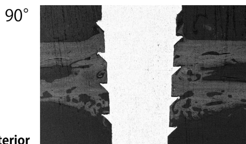
Fig. 7 Backscattered electron images of mini-implants at each insertion angle.
