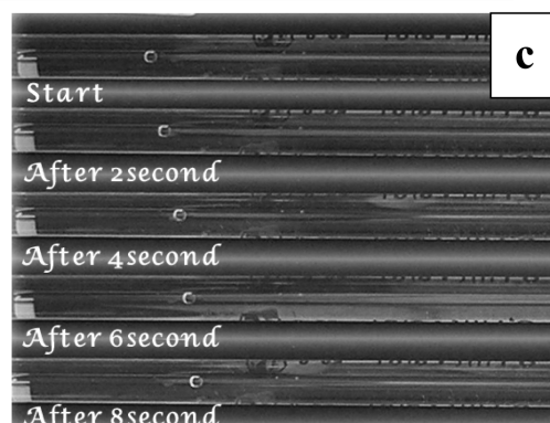
Fig. 1 (a) Schematic view of the designed fluid filtration system; (b) An enlarged view of the three-valve tube and its connections; (c) A typical picture of bubble movement.
