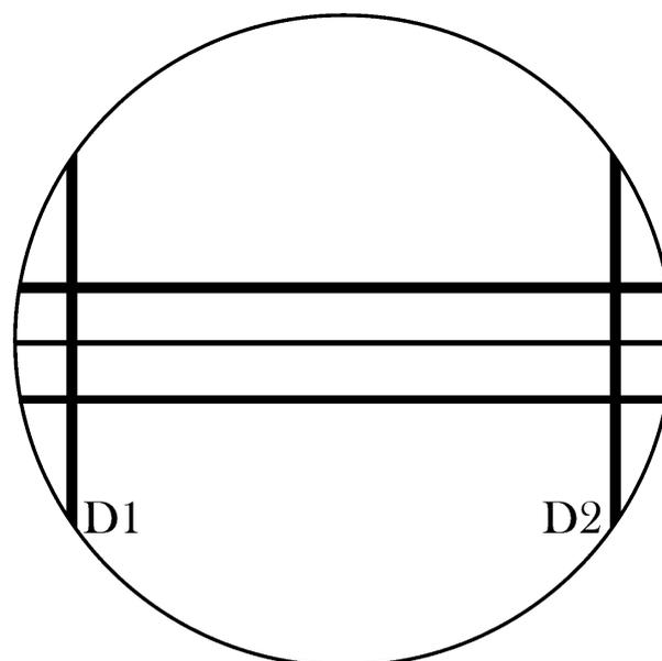
Fig. 1 Schematic illustration of the stainless steel test die showing the distance between the inner profile of Line d1 and the inner profile of Line d2 (d1-d2 distance). The width of vertical lines (d1 and d2) is  $0.075 \pm 0.008$  mm, whereas the distance between the lines d1-d2 is 25 mm.
