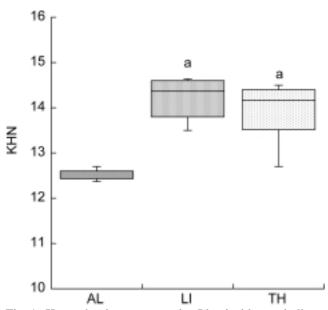
Fig. 1 Knoop hardness test results. Identical letters indicate that the values are not significantly different (P > 0.05).
