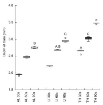
Fig. 2 Relation between curing depth and exposure period with the three photo-curing units. Identical letters indicate that the values are not significantly different (P > 0.05).
