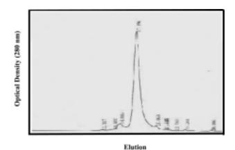
Fig. 3 Elution profile of the purified IgY fraction from r122k-HagA-immunized egg yolk using a gel filtration-HPLC column as described in the Materials and Methods.
